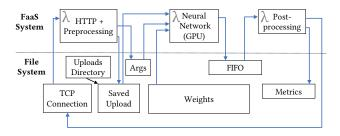
Figure 2: Model serving pipeline with separation of compute and state.
