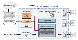
Figure 1: System Architecture of CloudEx
