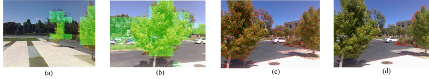
Figure 2: A feature selection example. (a)-(b) Results of classified regions with dense textures (masked in green). Note these regions mostly correspond to trees /leaves in the images. (c) The originally detected local features. (d) The remaining features after applying the region-sensitive feature selection.
