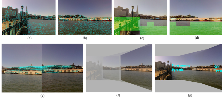
Figure 5: Results on a test sequence captured by the phone pilot system. (a)-(b) The detected feature points for panorama stitching, without feature selections. (c)-(d) The classified subregions with dense textures. For panorama, only a limited number of strongest features are selected from these regions. For image matching, we do not extract SURF features from these regions. (e) The result of feature point registration. Note that very few or none of the corresponding features come from regions with dense textures, which are hard to match and also very expensive for geometric verification using RANSAC. (f)-(g) Stitching the images into a panorama. (g) Panorama image after blending, with recognized points of interest labelled.
